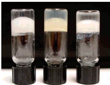
Figure 5. Selective organic liquid gelation over water (1/1 vol %). From left to right: paraffin oil, olive oil, and kerosene ( [1] = 26 \text{ mM} , 700 \mu\text{L} ) after 2 min sonication. The aqueous phase (top) is trapped by the gel.
